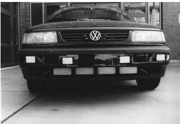
Fig. 4. Experimental vehicle equipped with a short range radar sensor network.
