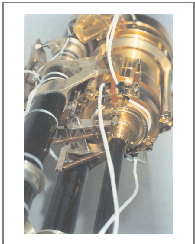
Fig. 5. The flight model of MUPUS insertion device in the stowed position on the lander balcony (right picture).
