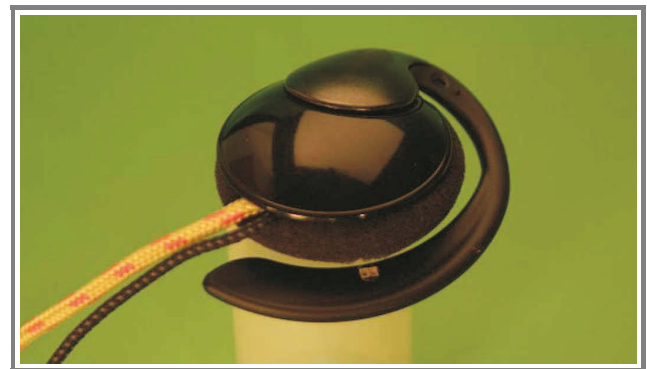
Fig. 6. Earphone-based sensor together with a recorder (© CSEM).
